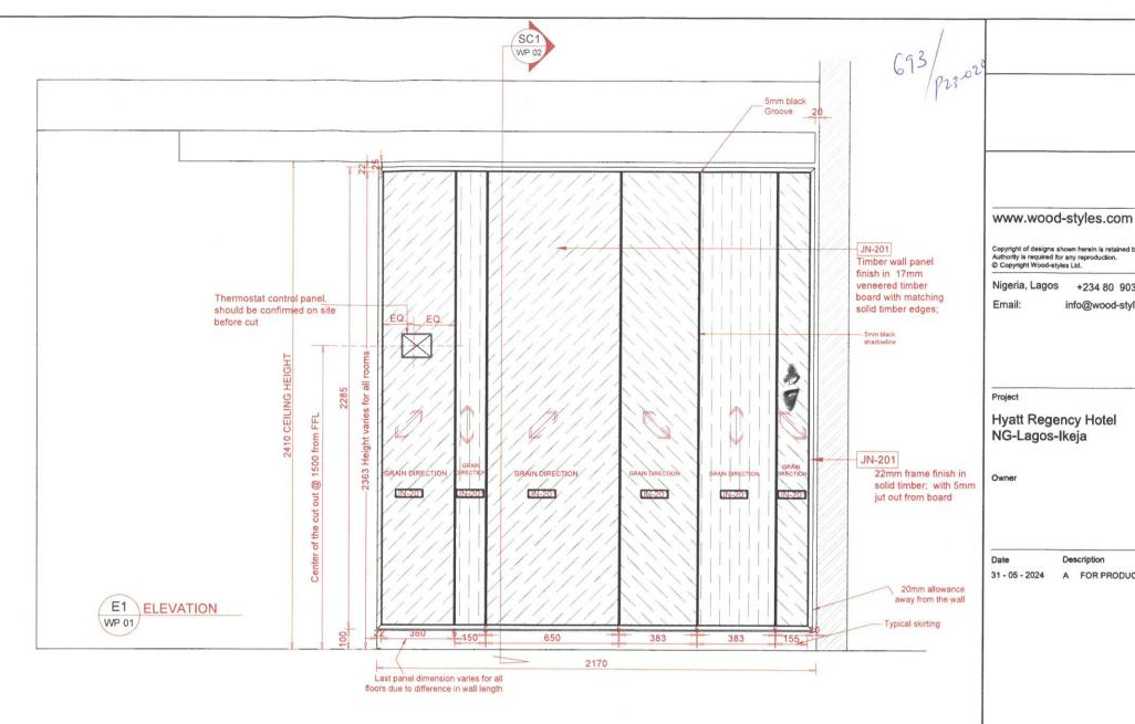
Cladding Position: Right side (Quantity: 12) (Face wall cladding) Note: Site dimension varies from room to room on the first floor
