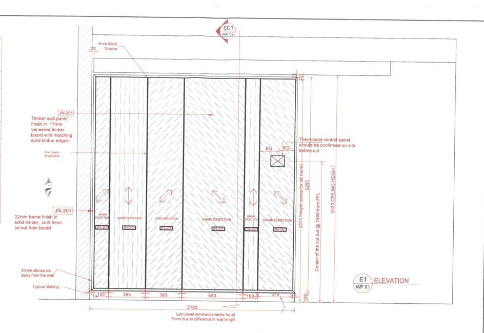
Cladding Position: Left side (Quantity: 10) (Face wall cladding) Note: Site dimension varies from room to room on the first floor
